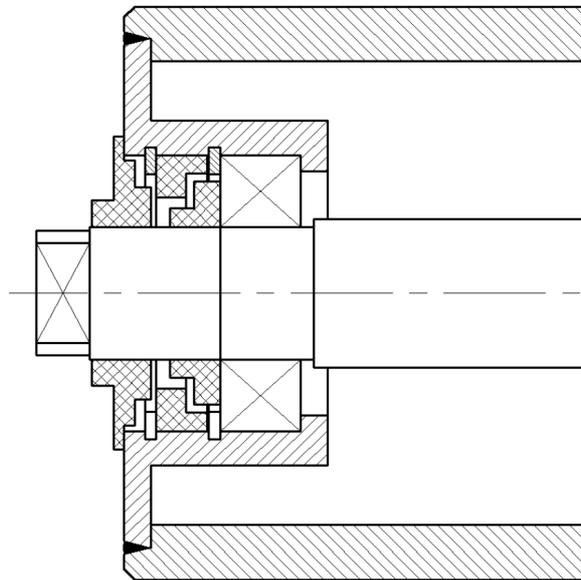
Fig. 4. Sealing system with simple labyrinth
