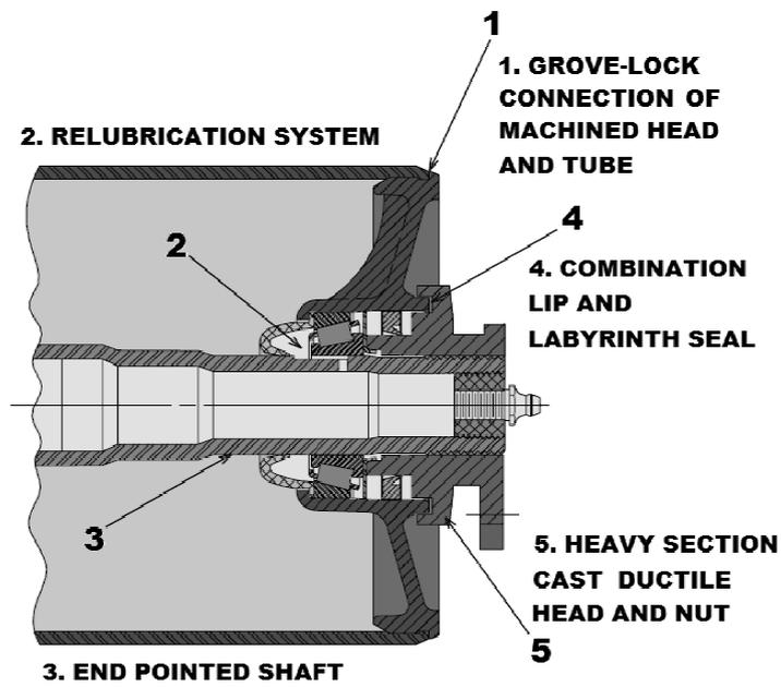
Fig. 6. SDX-Plus sealing system from Joy Mining Machinery
