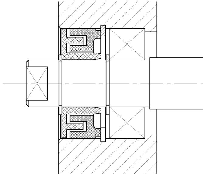
Fig. 5. Sealing system with double labyrinth
